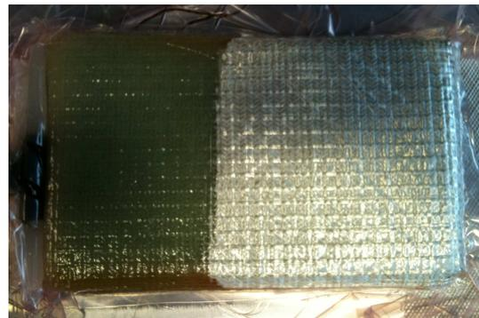
(c) Real image of the upper surface of one of the samples produced heating the resin. Linear flow front advance observed
