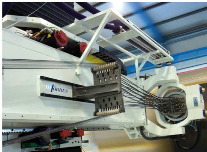
Figure 3.8: *Mtorres Fibre placement machine.*
