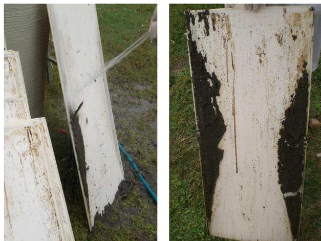
**Figure 6.5.** Images of cake formation on the membranes due to insufficient aeration.
