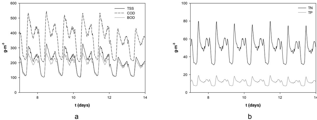
**Figure 5.2.** Influent wastewater organic matter (COD and BOD<sub>5</sub>) and TSS a) and nutrients (N,P) profile.
