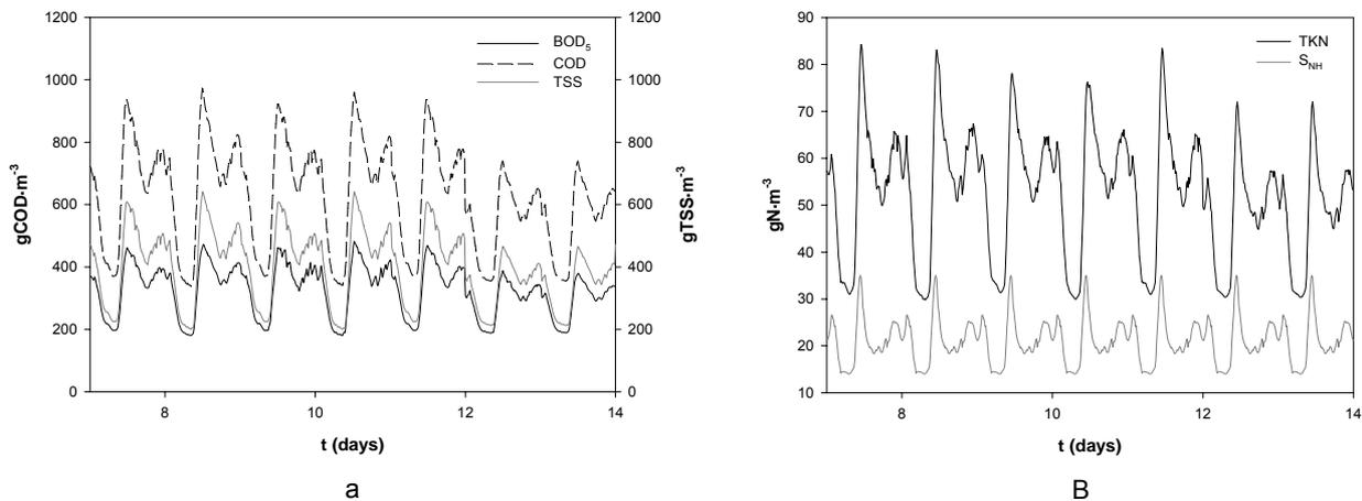
**Figure 7.2.** Influent wastewater a) organic matter (TSS, COD and BOD<sub>5</sub>) and b) nitrogen (TKN and ammonium) profile
