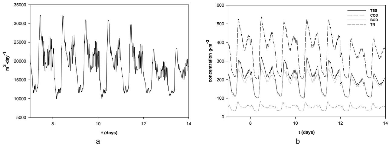
**Figure 4.3.** Influent wastewater flow (a) and components (b) profile
