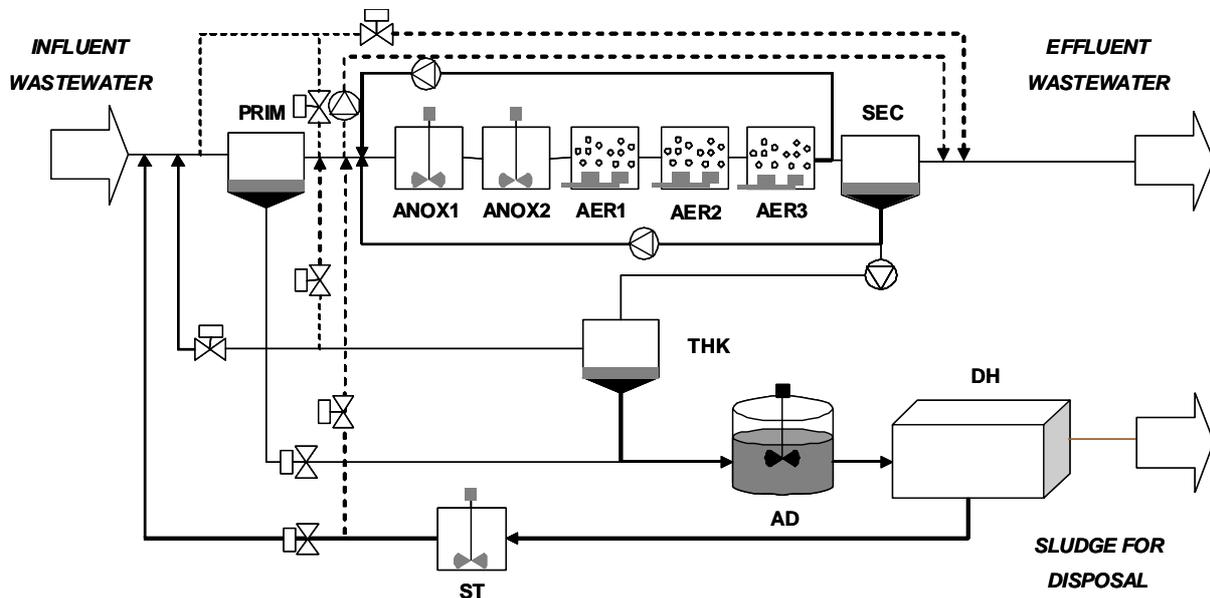
**Figure 6.2.** Plant layout for the BSM2 (Jeppsson *et al.*, 2006)
