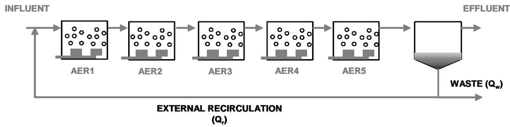
**Figure 4.2.** Flow diagram of the plant to be redesigned
