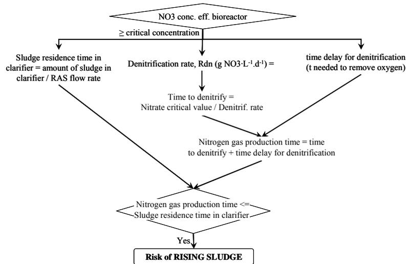
Figure A4.3. Flow diagram developed to evaluate the risk of rising sludge.
