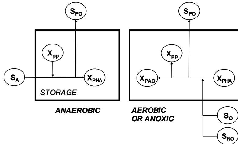
**Figure 3.2.** Illustration of the basic principles behind biological P removal as included in the ASM2d model (Gernaey *et al.*, 2004)
