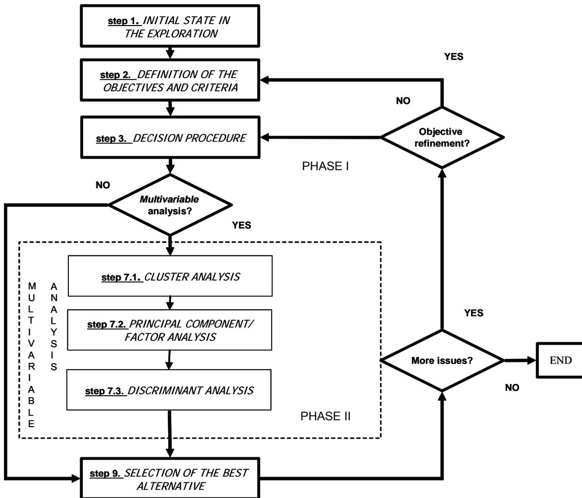
**Figure 6.1.** Flow diagram of the third block of the conceptual design method (see text for explanation)
