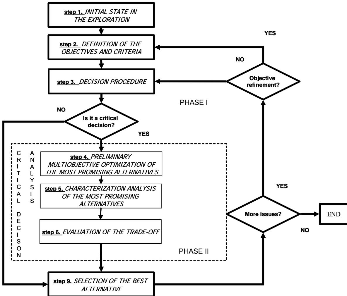
Figure 5.1. Flow diagram of the second block of the conceptual design method (see text for explanations).
