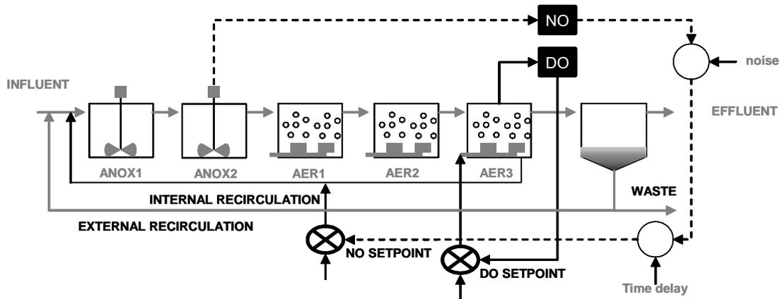
**Figure 4.7.** Schematic representation of the activated sludge plant with controllers
