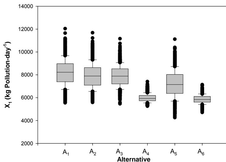
**Figure 7.4.** Effluent quality index ( $X_1$ ) variation using a multiple box plot representation.
