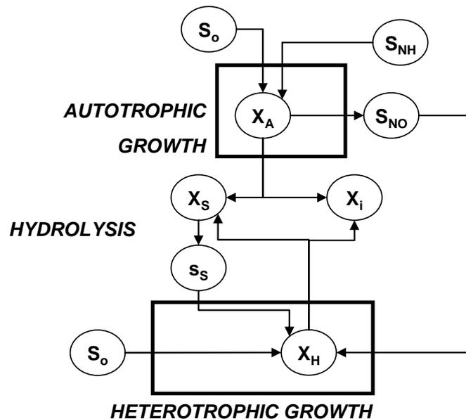
**Figure 3.1.** Substrate flow for autotrophic and heterotrophic biomass in ASM1 (Gernaey *et al.*, 2004)
