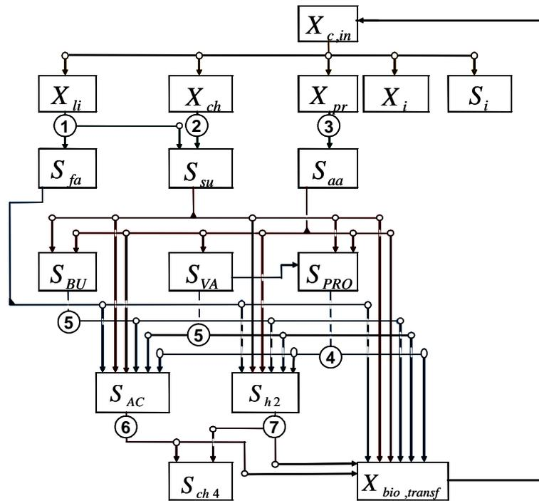
**Figure 3.5.** Representation of the biochemical reactions in the anaerobic digestion model (ADM1): (1) acidogenesis from sugars, (2) acidogenesis from amino acids, (3) acetogenesis from LCFA, (4) acetogenesis from propionate, (5) acetogenesis from butyrate and valerate, (6) acetoclastic methanogenesis and (7) hydrogenotrophic methanogenesis (from de Gracia *et al.*, 2007)
