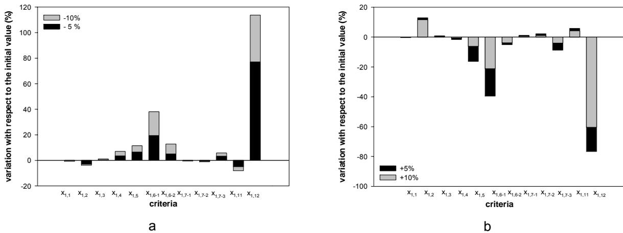
**Figure 5.3.** Variation of the evaluation criteria ( $x_{1,i}$ ) when the initial value of the anaerobic volume ( $V_{1,1}$ ) is decreased (a) and increased (b) respectively.
