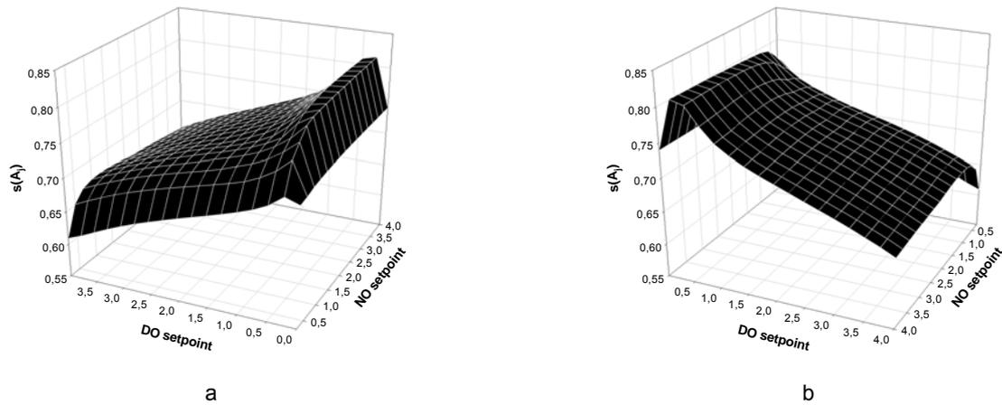
**Figure 4.12.** Two views of the multicriteria response surfaces generated using equation 4.1 ( $w_i = 0.25$ ,  $i = 1$  to 4)
