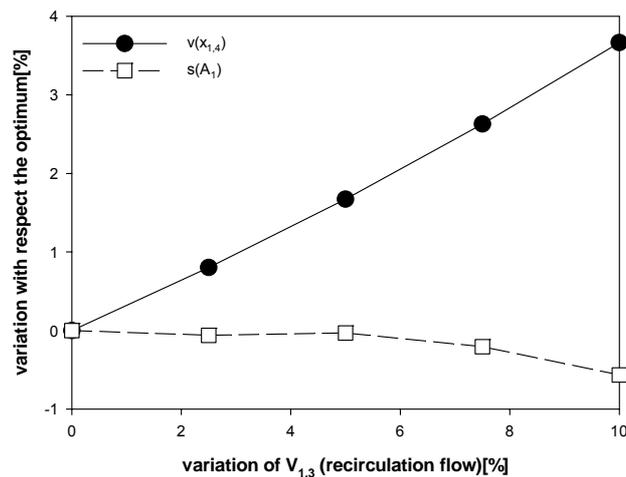
**Figure 5.10.** Trade-offs between the multiobjective function  $s(A_1)$  and the normalized value of criterion robustness  $x_{1,4}$ .
