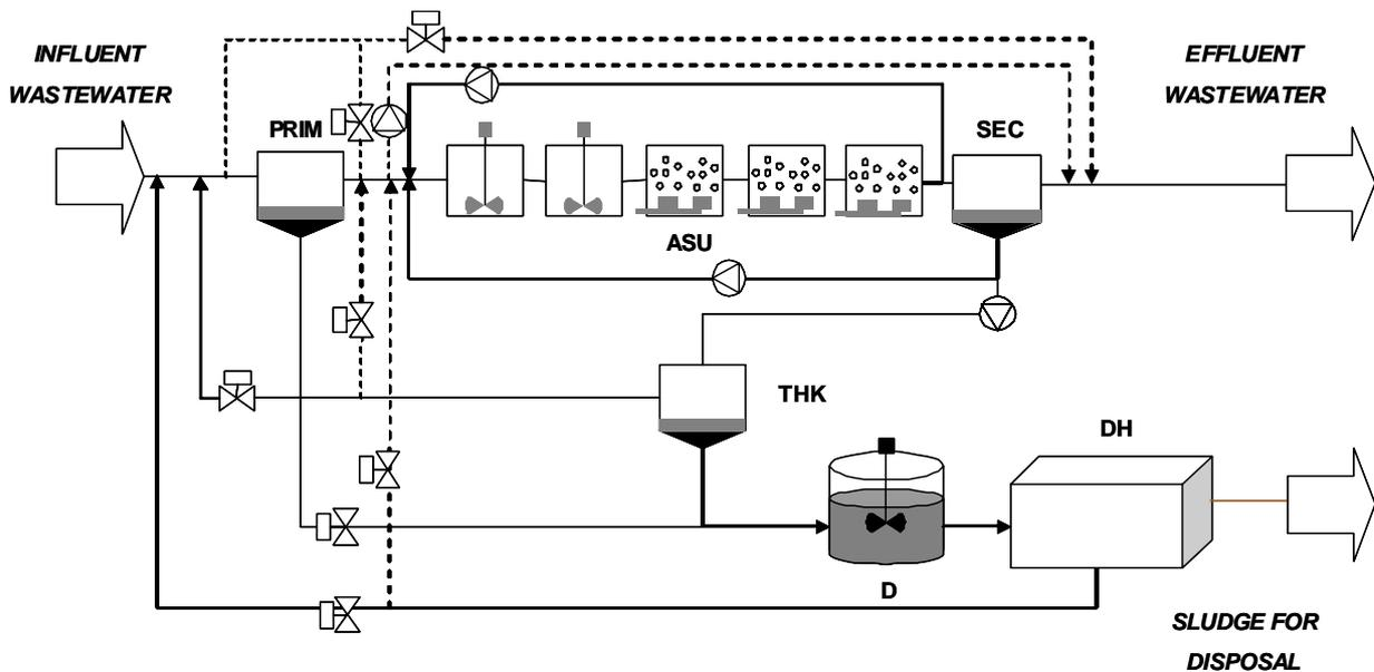
**Figure 3.3.** Flow diagram of a plant-wide WWTP
