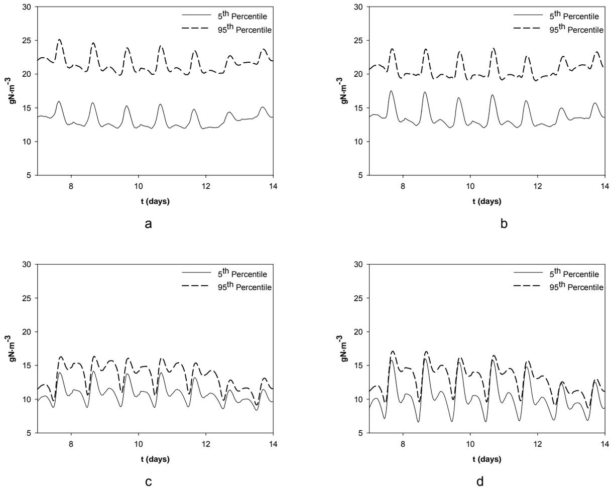
**Figure 7.8.** Dynamic uncertainty ranges for TN during the evaluation of alternative  $A_2$  (a),  $A_3$  (b),  $A_4$ (c) and  $A_6$  (d) under ASM parameters uncertainty. The TN profiles corresponding to the 5<sup>th</sup> and the 95<sup>th</sup> percentile resulting from the Monte Carlo simulations are shown.
