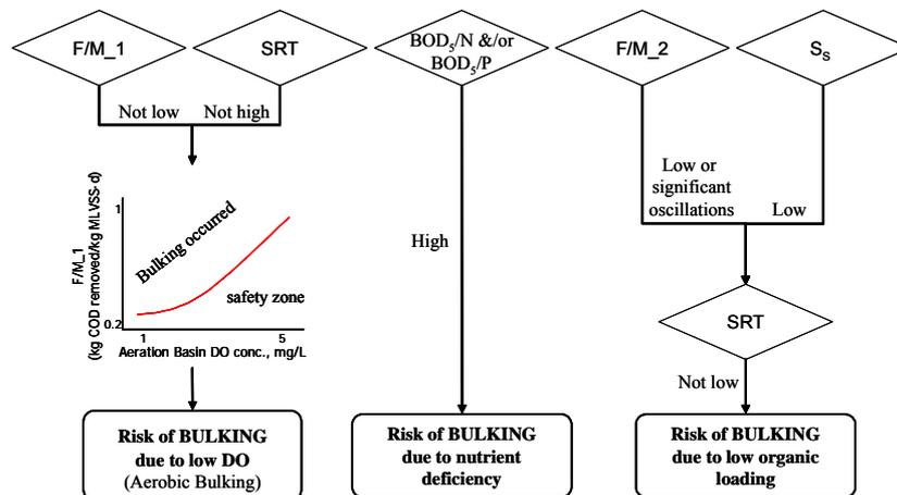
**Figure A4.1.** Flow diagram developed to evaluate the risk of filamentous bulking.
