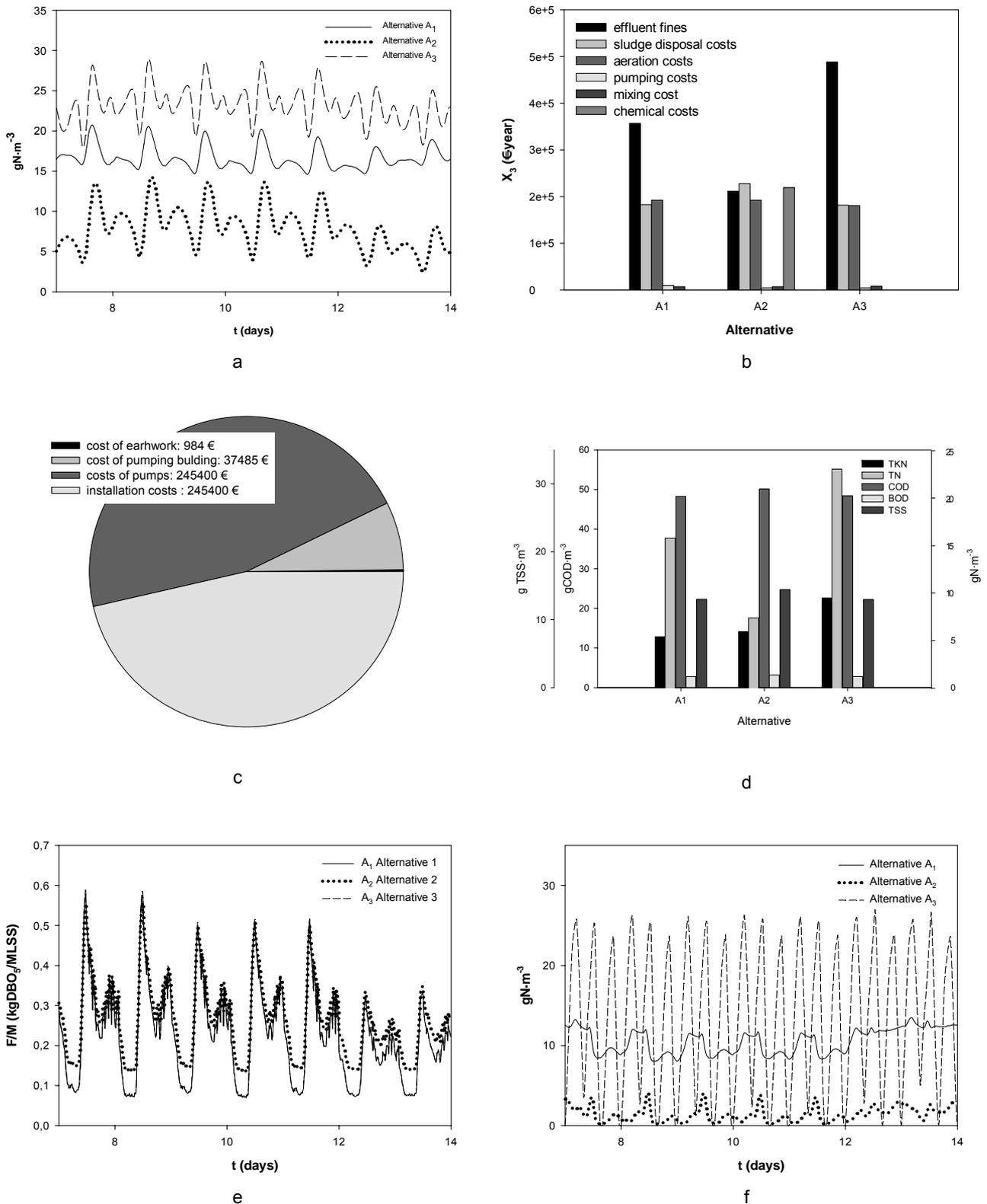
**Figure 4.4.** Representation of some of the evaluation criteria for the three alternatives evaluated: (a) dynamic effluent TN, (b) breakdown of operating costs, (c) pie chart of construction costs for alternative A<sub>1</sub>, (d) average effluent pollutant composition (e) F/M ratio and (f) effluent nitrate composition
