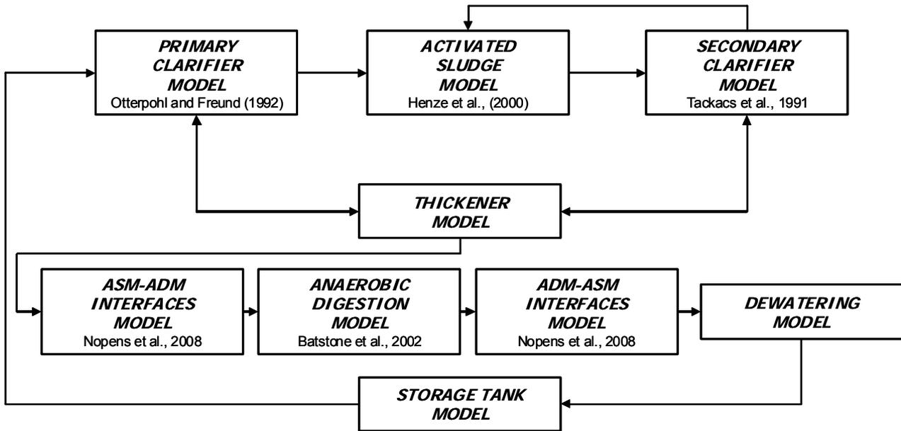
Figure 3.4. Schematic representation of the different models at plant wide level
