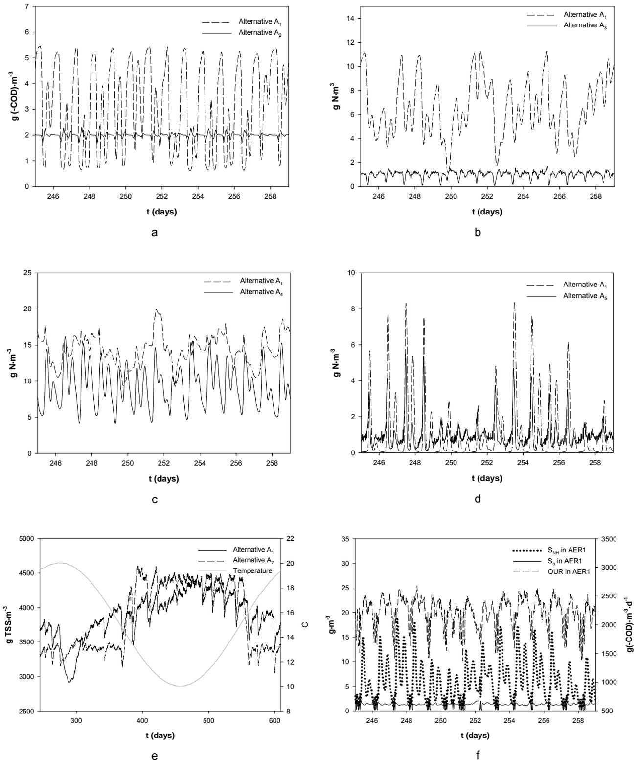
**Figure 6.4.** Behaviour of the different controllers studied: (a)  $S_0$  controller, (b)  $S_{NO}$  controller by means of the manipulation of  $Q_{intr}$ , (c)  $S_{NO}$  controller by means of manipulation of  $Q_{carb}$ , (d)  $S_{NH}$  controller, (e) TSS controller and (f) OUR controller
