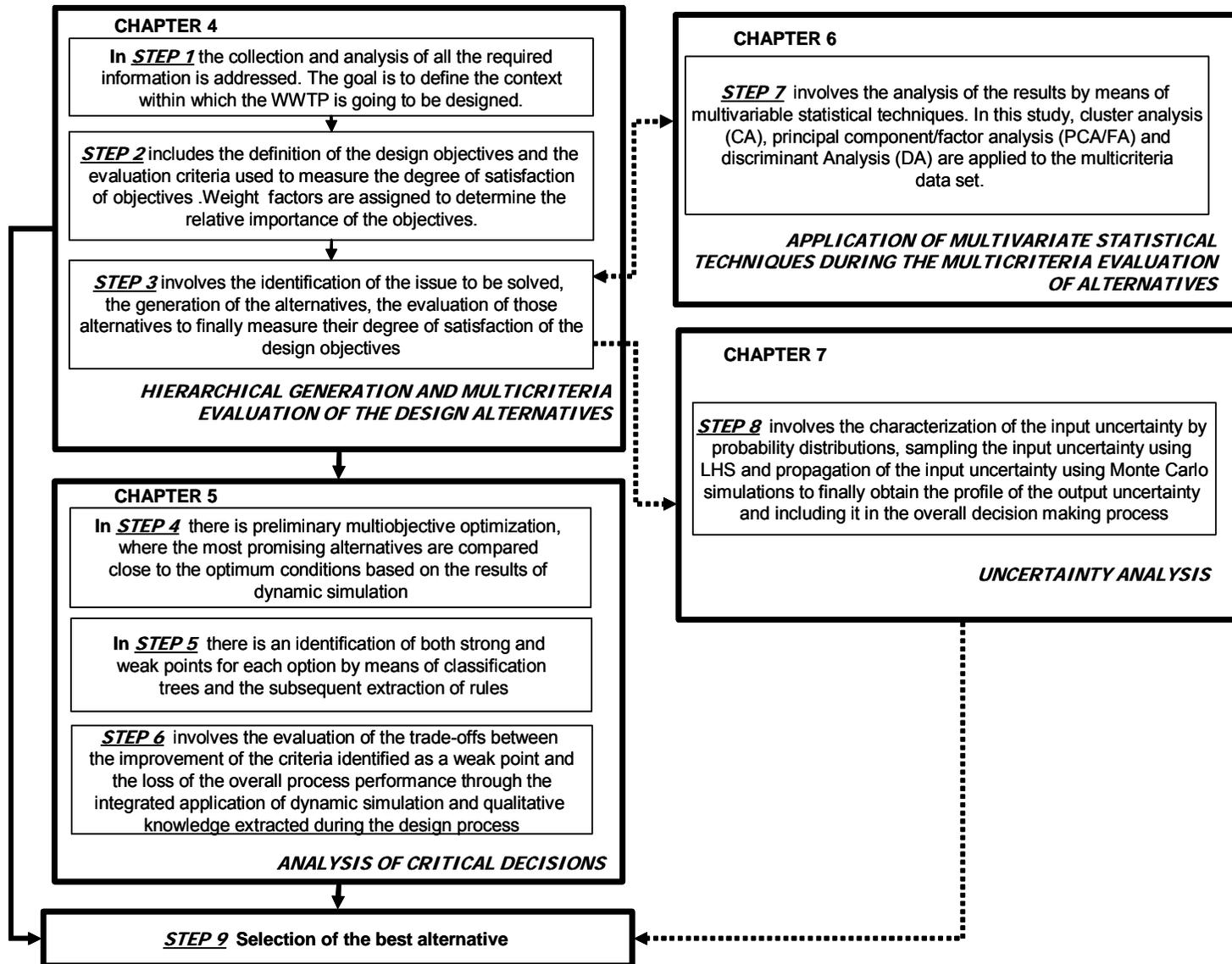
Figure 2.1. Simplified structure of the proposed conceptual design method (see text for explanations)
