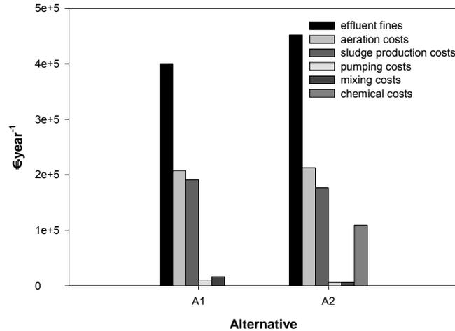
**Figure 5.9.** Breakdown of the operating costs ( $X_3$ ) for the most promising alternatives.
