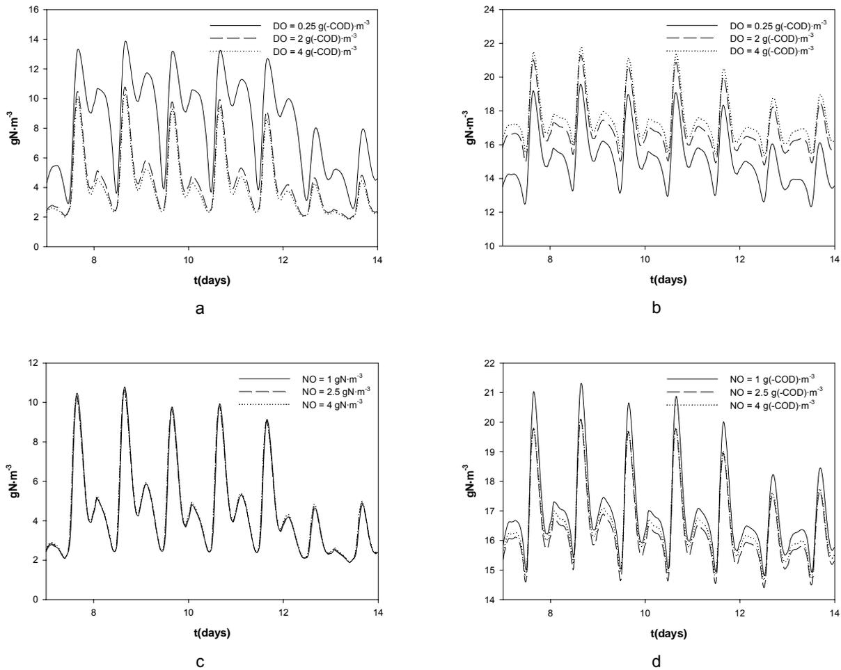
**Figure 4.9.** Dynamic profiles of both TKN (a,c) and TN (b,d) for different set point combinations (a – b) when the NO set point is constant ( $\text{NO} = 1 \text{ g N}\cdot\text{m}^{-3}$ ) and the DO set point is changed; and (c-d) when the DO set point is constant ( $\text{DO} = 2 \text{ g (-COD)}\cdot\text{m}^{-3}$ ) and the NO set point is changed.
