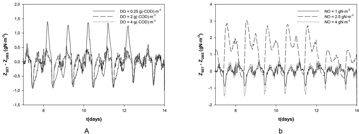
**Figure 4.10.** Dynamic profiles of the difference between the nitrate in the second anoxic reactor ( $Z_{OBS}$ ) and the desired set point ( $Z_{SET}$ ) for different set point combinations a) when the NO set point is constant ( $\text{NO} = 1 \text{ g N}\cdot\text{m}^{-3}$ ) and DO is changed and b) when the DO set point is constant ( $\text{DO} = 2 \text{ g}(-\text{COD})\cdot\text{m}^{-3}$ ) and NO is changed
