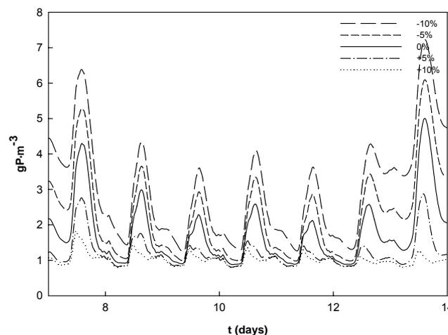
**Figure 5.5.** Evolution of the total phosphorus concentration in the effluent for the different scenarios: alternative  $A_1$  analysing the variable ( $V_{1,1}$ ).
