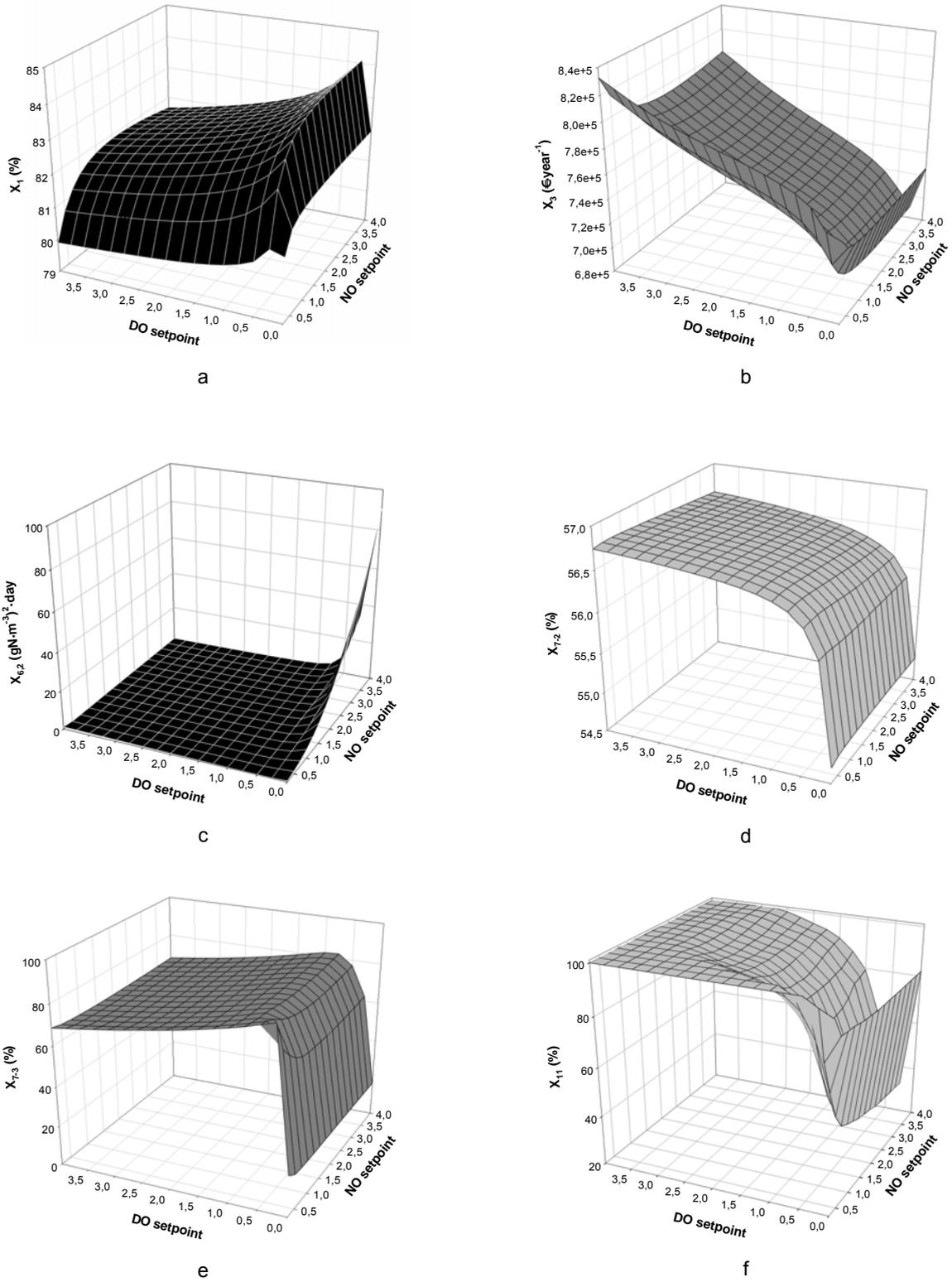
**Figure 4.8.** Representations of some of the evaluation criteria: (a) impact on water ( $X_1$ ), (b) operating costs ( $X_3$ ), (c) nitrate control performance ( $X_{6,2}$ ), (d) foaming risk, (e) rising risk ( $X_{7,3}$ ) and (f) time in violation (TIV) for TN ( $X_{11}$ )
