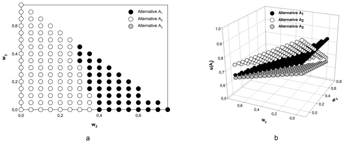
**Figure 4.6.** Sensitivity analysis of  $w_2$ ,  $w_3$  and  $w_4$  (a,b)
