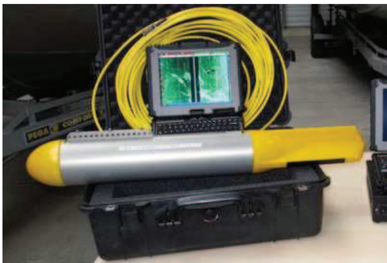
Figura 4.1: Torpede Imagenex model 782 "Yellowfin", cable i ordinador.
