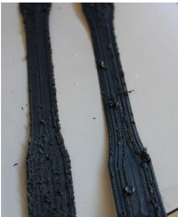
Figure 22 Printing was not possible with bigger thickness
