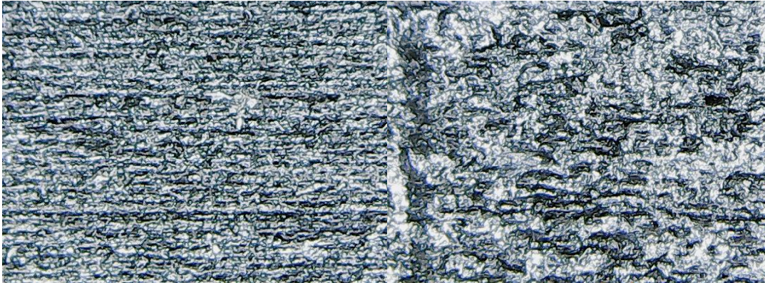
Figure 28-29 Surface of the third type of specimen from CF-ABS, before and after acetone treatment
