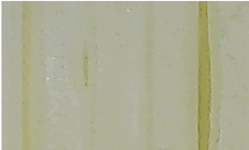
Figure 20 Voids between the lines
