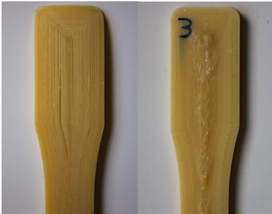
Figure 13 Example for weak connection between the lines and for using too much material
