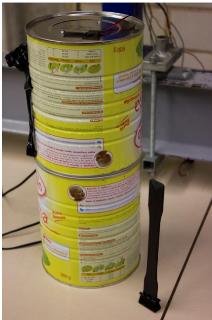
Figure 24 Equipment for acetone surface treatment
