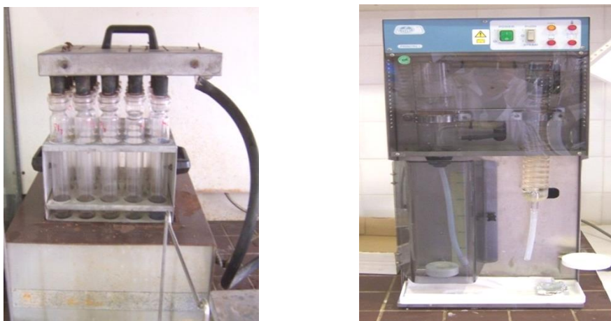
Figure 20. The digestion and distillation units used for the determination of total nitrogen.
