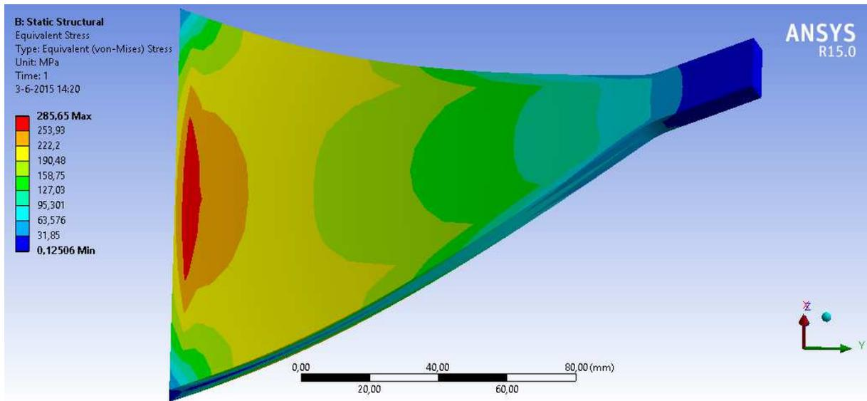
Figure 23: ANSYS Workbench: equivalent (von-Mises) stress
