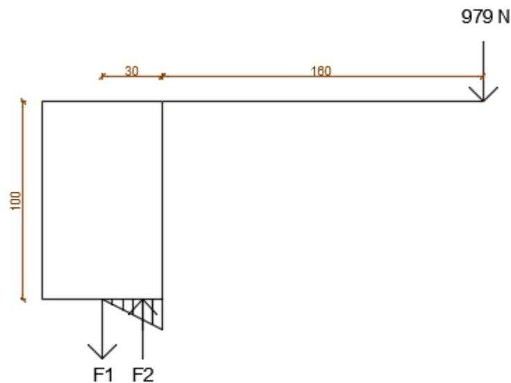
Figure 17: Sketch of the calculation of the required tensile strength
