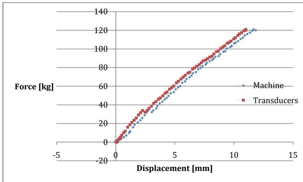
Figure 29: Force–displacement graph
