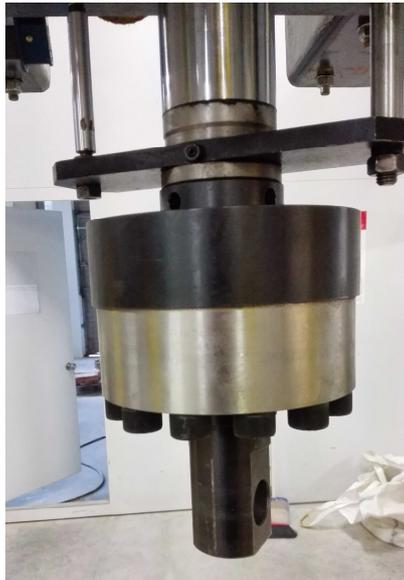
Figure 8: Ending of the piston, provided with a load cell of 300 kN of capacity
