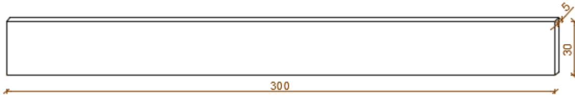
Figure 6: Design tensile specimen
