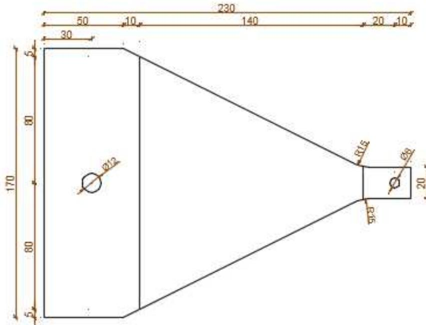
Figure 16: Final geometry TADAS-specimen
