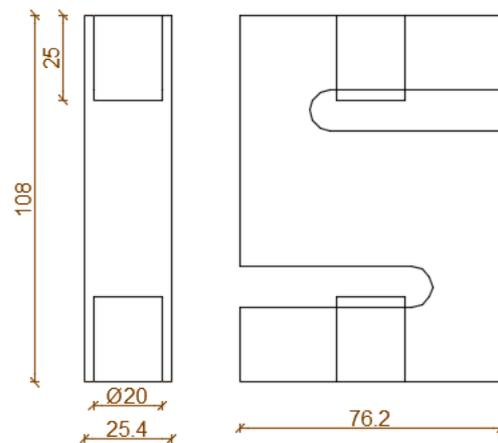
Figure 42: Load cell MODELO 630
