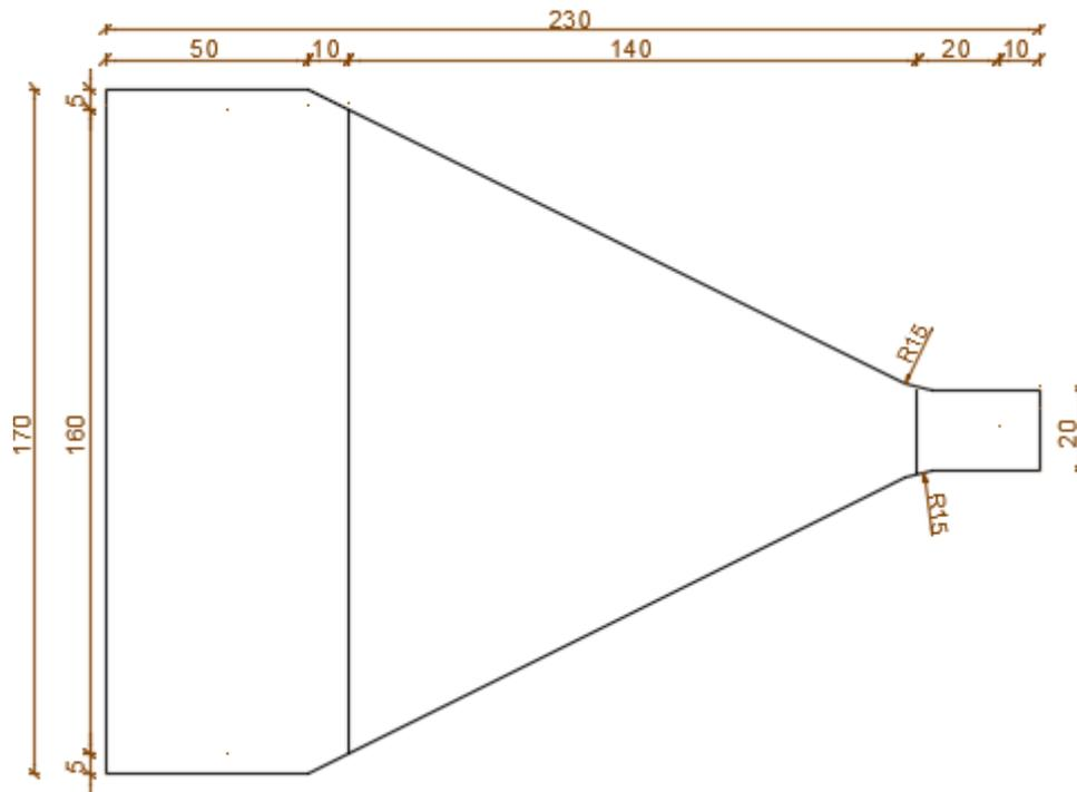
Figure 5: First design TADAS-specimen
