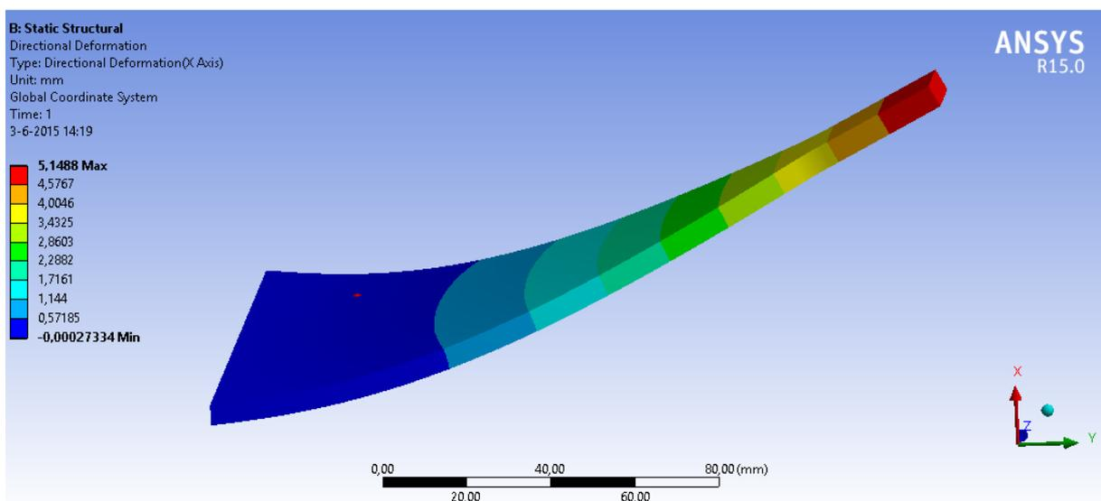
Figure 22: ANSYS Workbench: directional deformation
