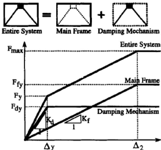
Figure 1: Schematic hysteretic behavior of structures with hysteretic dampers (Nakashima, Saburi, & Tsuji, 1996)
