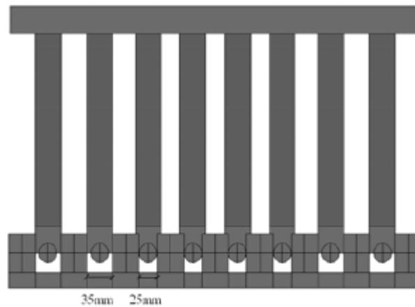
Figure 38: Modified-TADAS Configuration (Dareini & Hashemi, 2011)
