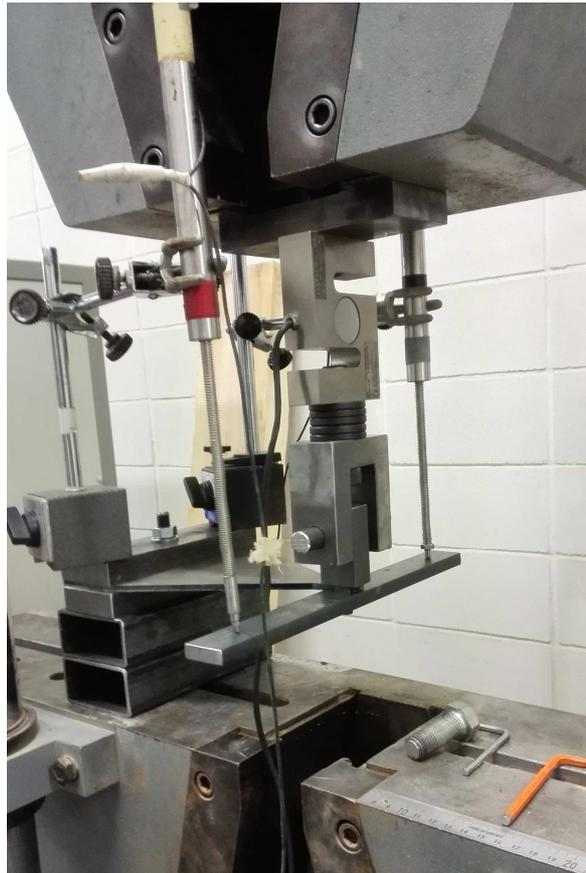
Figure 25: Mounting of displacement transducers LVDT/150/01
