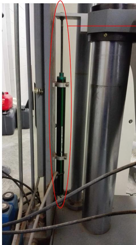
The displacement of the piston of the machine is measured by this appliance
