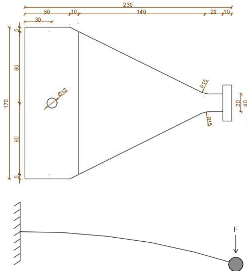
Figure 35: Proposal geometry TADAS–specimen for future design
