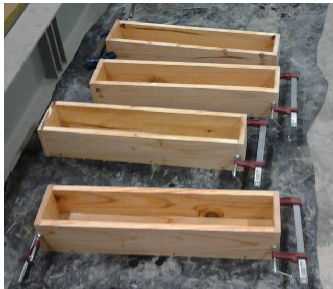
Fig 4-21 - Wooden moulds for the first concrete type (600x100x100mm)
