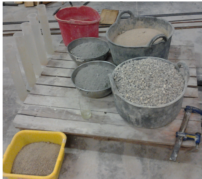
Fig 4-17 - Preparation of the concrete ingredients
