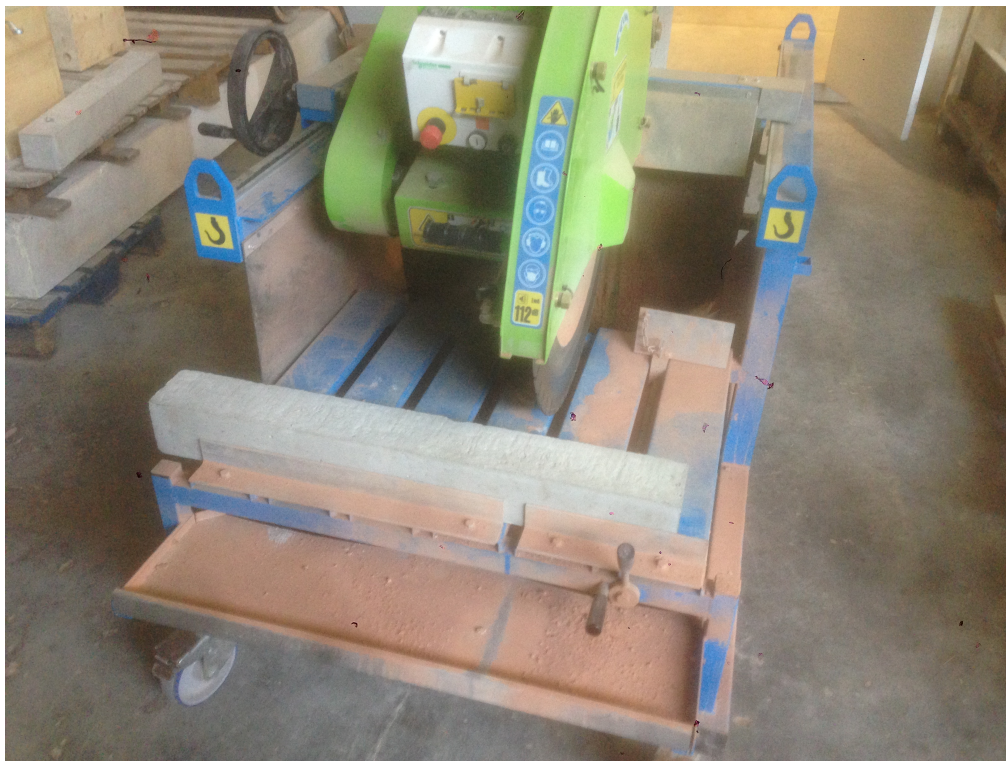
Fig 4-18 - Wet cutting of the trial specimens to length
