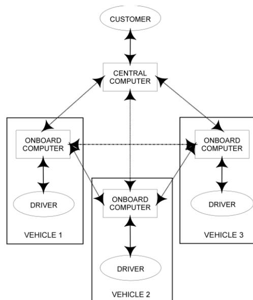
Figure 3 - Schematic of Communication in ADART (Dial, 2003)
