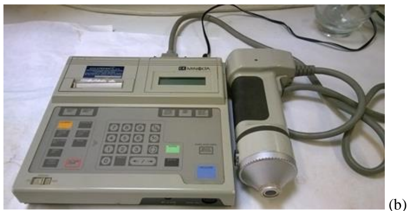
Figure26: “a” schema and “b” Colorimeter
