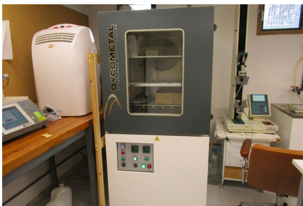
Figure 3.3.8: Climatic chamber for samples conditioning
