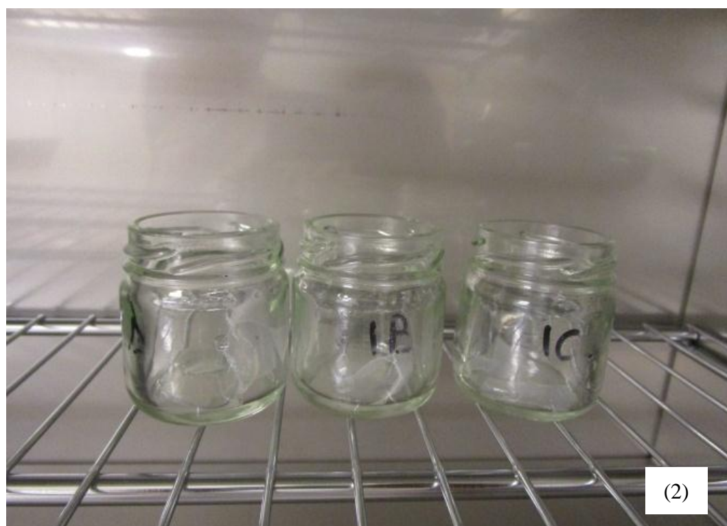
Figure 3.5.3 (c): Biodegradability testing (1) samples were put in the oven at 50°C and (2) samples were dried in the oven at 50°C after filtration
