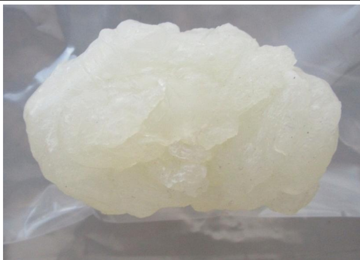
Figure 3.4.4 (b): Obtained blend after Brabender mixing
