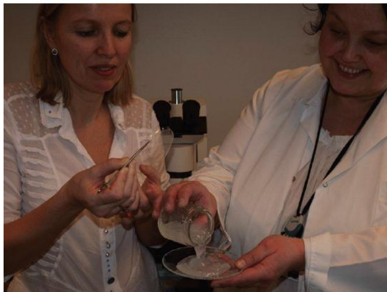
Figure 1.10.4 (b 1 ): NFC film and 0.4% consistency NFC gel produced at the Paper and Fiber Research Institute (PFI), Trondheim, Norway, being handled by Kristin Syverud (left) and Ingebjorg Leirset (right) [88]
