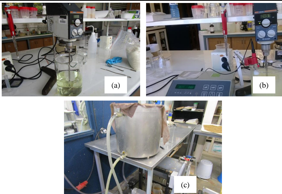
Figure 3.3.10: Equipment for oxidized pulp preparation (a) mixer, (b) pH meter, and (c) vacuum filtration machine
