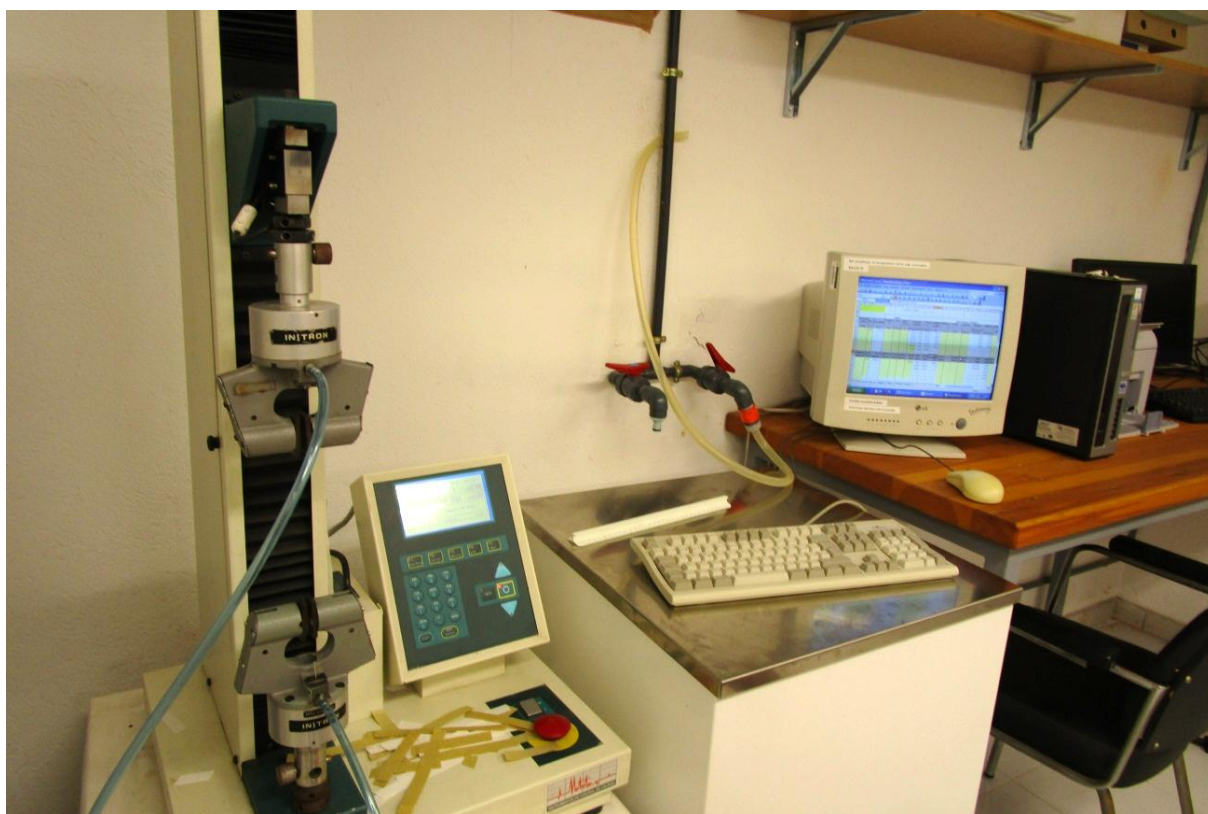
Figure 3.3.9: Tensile testing machine with 2.5kN of load cell
