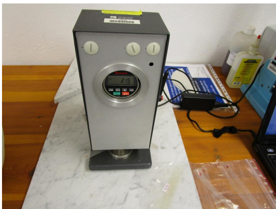
Figure 3.4.8: Films' thicknesses measurement procedure
