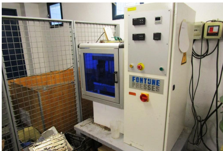
Figure 3.3.3: Thermoforming, compression machine
