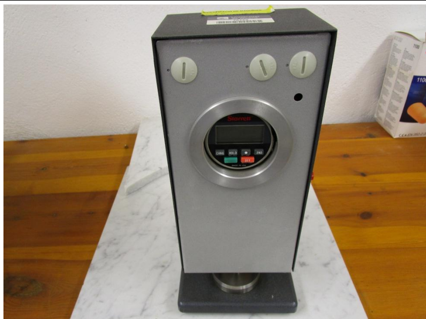
Figure 3.3.7: Machine for films' thicknesses measurement
