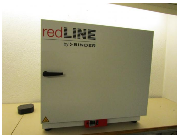
Figure 3.3.14: Drying oven for water uptake and biodegradability testing of films
