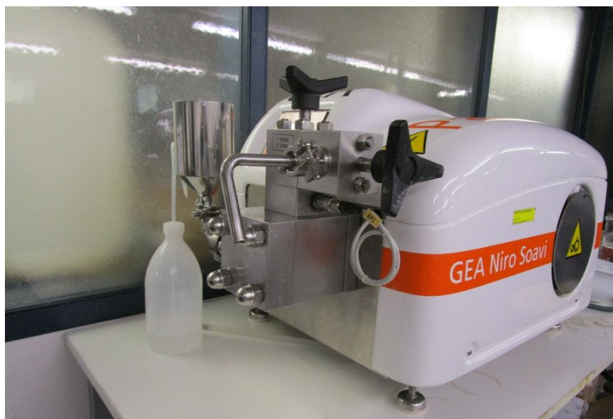
Figure 3.3.12: Homogenizer for NFC preparation
