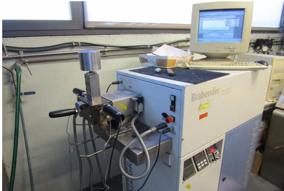
Figure 3.3.2: Brabender mixer, mixing machine
