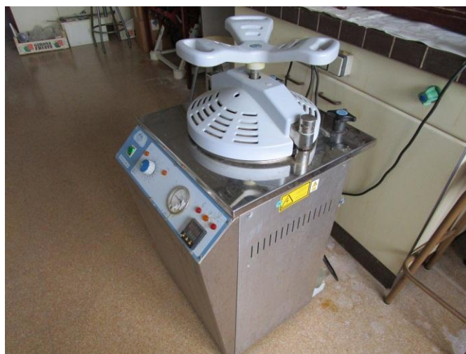
Figure 3.3.15: Autoclave for bottles sterilization
