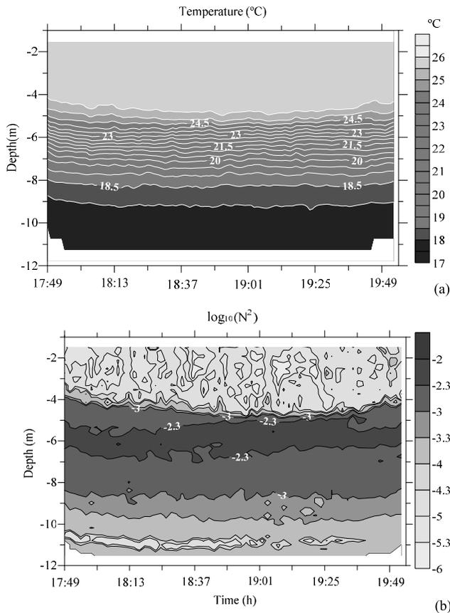
**Figure 3.** The contour plot of (a) temperature  $T$  and (b) logarithm of squared buoyancy frequency  $\log_{10}N^2$  for June 25 ( $N$  is in  $s^{-2}$ ).
