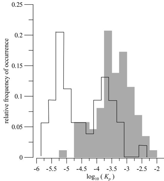
**Figure 13.** The histogram of the logarithm of turbulent diffusivities in microstructure patches for July 1 (gray bars) and June 25 (open bars).
