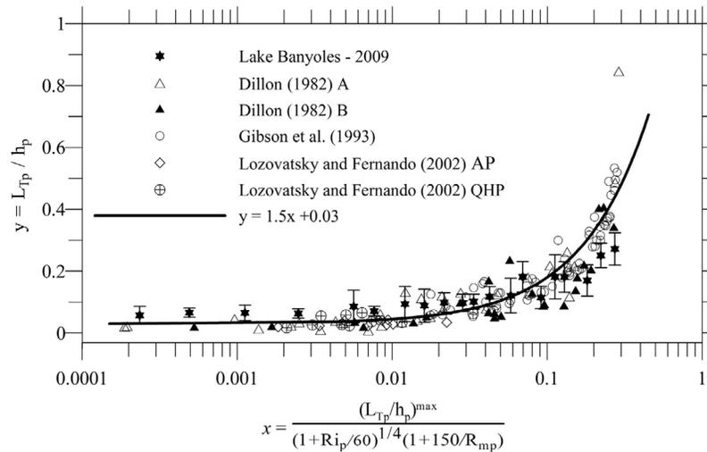
**Figure 11.** The normalized patch Thorpe scale  $L_{Tp}/h_p$  as a function of the patch Richardson  $Ri_p$  and mixing Reynolds  $R_{mp}$  numbers (see text for details).
