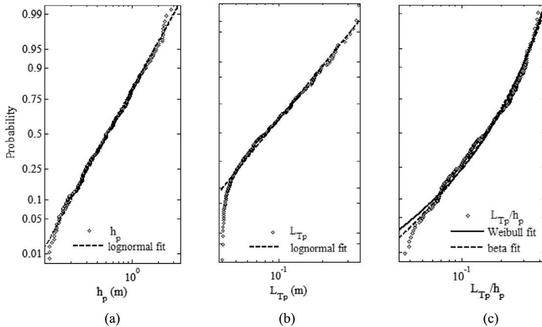
**Figure 10.** The cumulative distribution functions (CDF) of (a) the patch sizes  $h_p$  in the thermocline and (b) the patch Thorpe scale  $L_{Tp}$  fitted by lognormal model (dashed lines). (c) The CDF of the normalized patch Thorpe scale  $L_{Tp}/h_p$  is approximated by the Weibull (solid line), and beta (dashed line) distributions.
