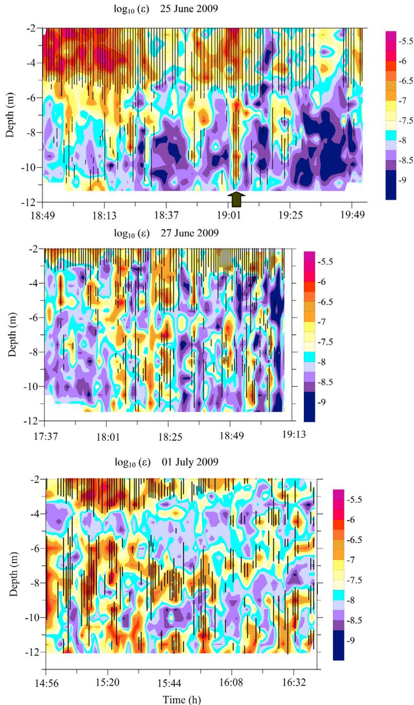
**Figure 6.** Alignment of microstructure patches (vertical lines) in the background of  $\log_{10} \varepsilon$  for (top) June 25, (middle) June 27 and (bottom) July 1. The dissipation rate is in  $\text{W kg}^{-1}$ . The arrow in Figure 6 (top) points to the turbulent event induced by the wind gust.
