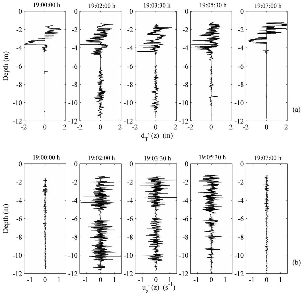
**Figure 9.** A series of (a) Thorpe displacements  $d_T'(z)$  and (b) small-scale shear  $u_z'(z)$  profiles taken on June 25 during the passage of a wind gust (see text for details).
