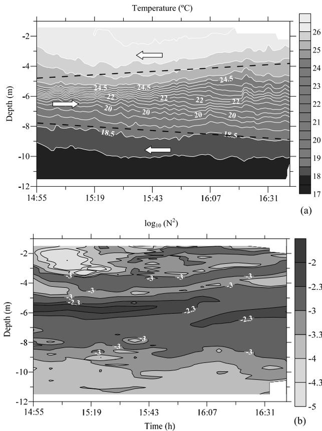
**Figure 5.** The contour plot of (a) temperature and (b)  $\log_{10} N^2$  for July 1. The opposite slopes of the upper and lower boundaries of the thermocline marked by dashed lines point to the dominant second mode of the internal seiche. The directions of flow in each layer are shown in Figure 5a by white arrows.
