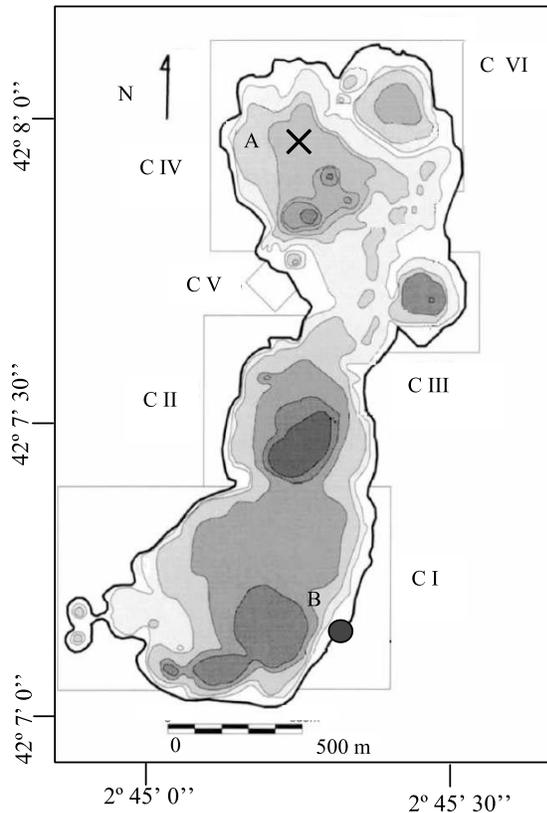
**Figure 1.** Bathymetric map of Lake Banyoles [from Moreno-Amich and Garcia-Berthou, 1989]. With kind permission from Spring Science+Business Media. Distance between the isobaths is 5 m. The main basins (C-I to C-VI) are shown on the map. Point A indicates the measurement site and point B the location of the meteorological station.
