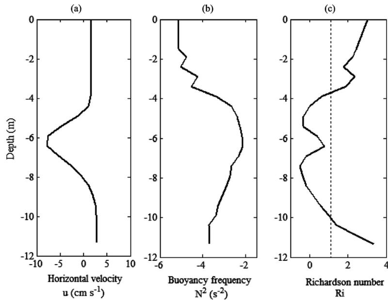
**Figure 7.** (a) The horizontal velocity profile of the second vertical mode of internal seiche  $u$  calculated for (b) a characteristic  $N^2$  profile and (c) the resulting profile of  $\log_{10} Ri$ .
