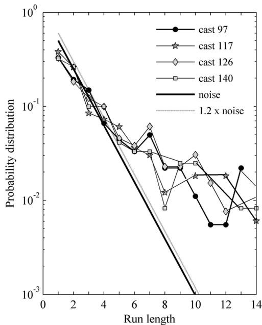
**Figure 2.** The probability density functions of the Thorpe run lengths for different profiles. The pdfs of random, uncorrelated noise (thick line) and of the noise factor 1.2 (dashed line). The intersection between the measured and noise pdfs indicates the cutoff run length equals 5.
