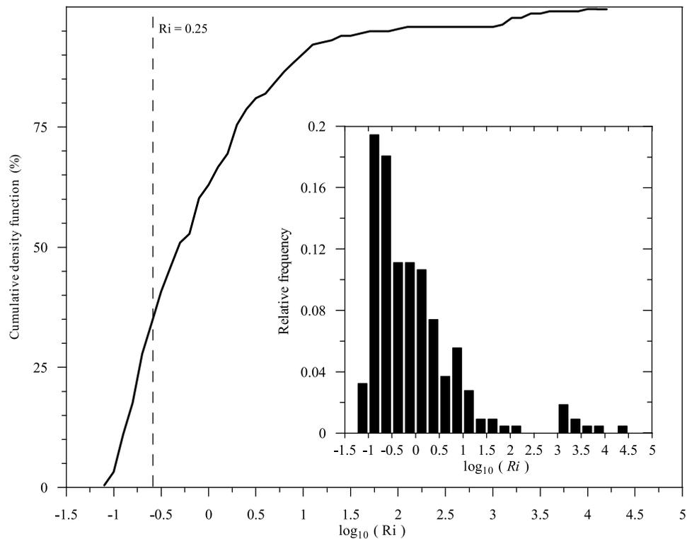
**Figure 8.** The cumulative distribution function (CDF) of the simulated seiche Richardson numbers  $Ri$  in the thermocline. The histogram of  $Ri$  is in the insertion.
