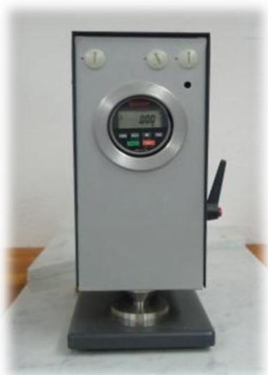
Figure 4.13. Micrometer
