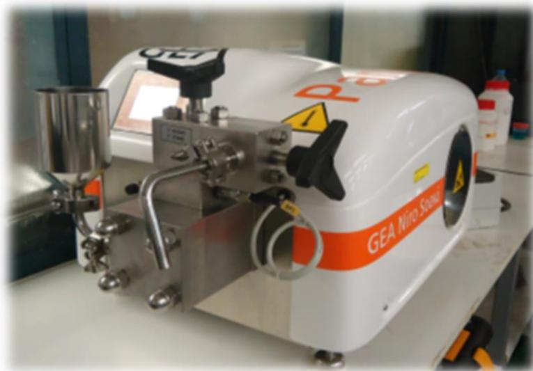
**Figure 4.5. Homogenizer**
