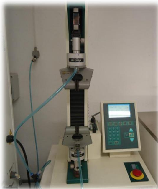
Figure 4.16. Hounsfield Instron dynamometer
