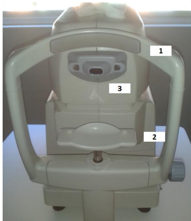
1. Forehead bar 2. Chin rest. 3. Puff of air exit and beam of light exit and entrance (pneumatic system and optoelectronic applanation monitoring system)
