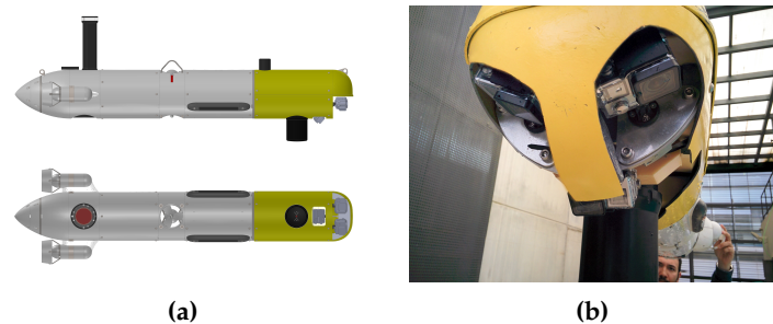
Figure 13. Sparus II AUV. (a) CAD model, where the three thrusters can be observed, as well as the profiling sonar and cameras located in the payload area (yellow); (b) real-world vehicle's payload.
